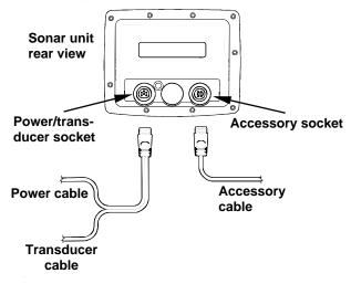
Sonar unit cable connections.
